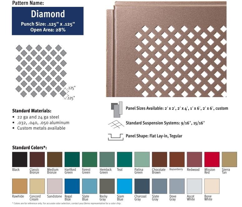
**Finishes:** Materials are pretreated, primed and, roller-coil coated with a 1.0 mil total dry film thickness (.2 mil primer with a .8 mil topcoat). The reverse side is coated with a wash coat of .4 to .5 mil dry film thickness.
