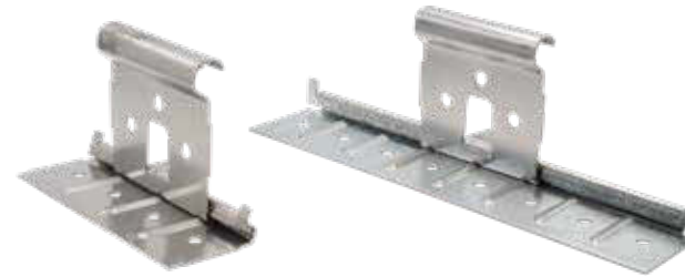
BEMO Hook Clip to accommodate metal panels as long as 328' (100 m). BEMO Long-slide Hook Clip with 7.5" (190 mm) of travel to accommodate metal panels as long as 400' (122 m).
