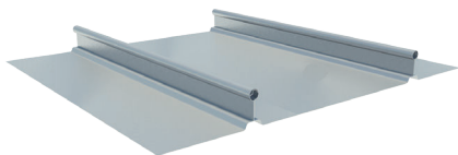
Standing round seam profile Aluminum min. 0.9 mm (19 gauge) Steel min. 0.75 (22 gauge)
