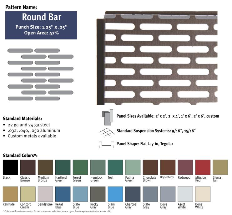
**Finishes:** Materials are pretreated, primed and, roller-coil coated with a 1.0 mil total dry film thickness (.2 mil primer with a .8 mil topcoat). The reverse side is coated with a wash coat of .4 to .5 mil dry film thickness.
